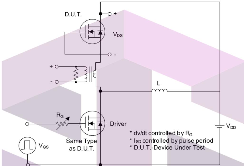
Fig. 1.1 Peak Diode Recovery  $dv/dt$  Test Circuit
